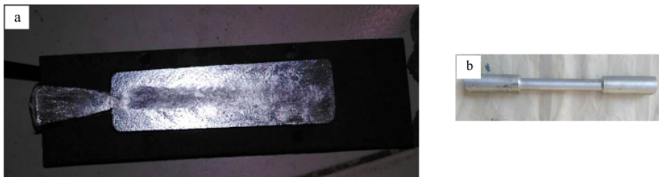
Figure 1.(a) Casting product of Al10Si-xCu (b) Specimen of tensile test after machining
